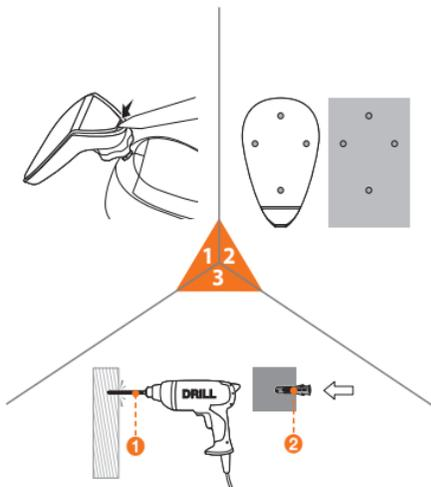
Place the bracket cover against the wall where the camera will be mounted and mark the position of the screw holes.
