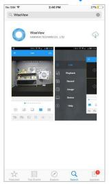
2. Open WiseView, and go to Device. Click 'to add new device. Scan QR code under Information page of system on local NVR. Then input client port, user name and password, and then click Save to log in the device.
