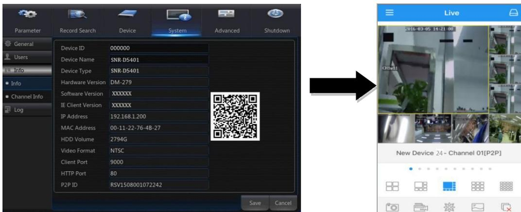
It supports max. 1080P resolution during live view on mobile phones. If the image resolution is above 1080P, the video will not be fluent.
