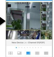
It supports max. 1080P resolution during live view on mobile phones. If the image resolution is above 1080P, the video will not be fluent.
