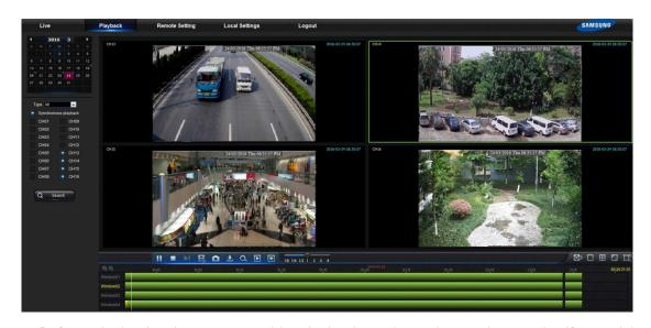
Before playback, choose to enable playback 4 channels synchronously. If you tick-select "Synchronous playback", that means the selected channel will playback synchronously; otherwise, you could separately control the channels playback.
