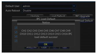
**Note:** Do not take out the USB memory or turn the power off during upgrading. When the update is done, system will be automatically restarted. After about 5 minutes, the upgrading will be finished. It is recommended to load ex-factory default after upgrading. The auto maintain function can be effective only when the NVR returns back to Preview mode with no any operation within the set auto maintain time.
